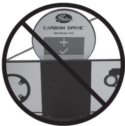
Figure 2: Tension excessive de la courroie
